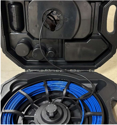
Fig. 49 : Incorrect: Camera cable not pulled taut
