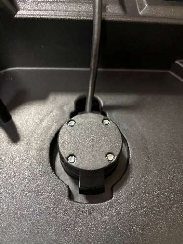
Fig.48 : Insert the camera cable into the upper shell and pull it tight carefully
